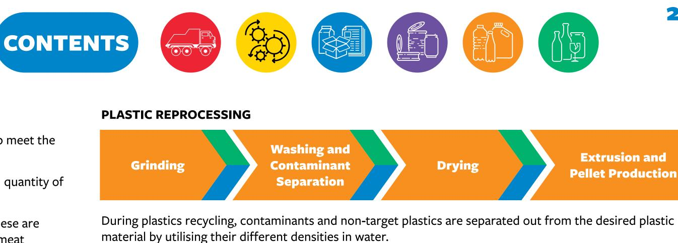
Water has a density of 1g/cm<sup>3</sup>, therefore in order to separate plastics from each other you are dependent on the ability of some of those plastics to float in water and some to sink.
