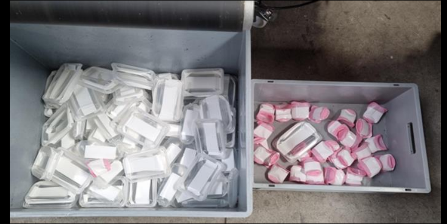
With UV – select INJ packs (Yield 97%, purity 97%) Extrusion packs not selected (Yield 98%, purity 98%)
