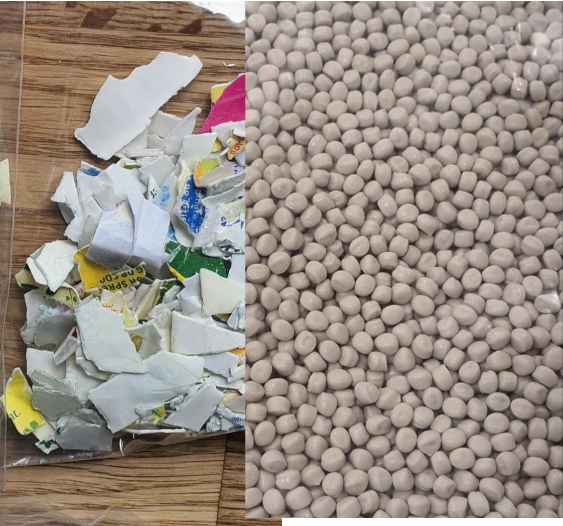
Recycling with IML labels left on
